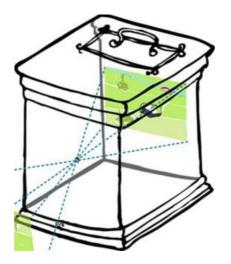
Light waves enter through this hole and hit the surface opposite the hole. This way, an image is projected onto the opposite surface, which acts as a screen.
